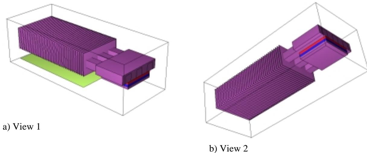
Figure 1 Coolit model of TEC & heat pipe cooling system
